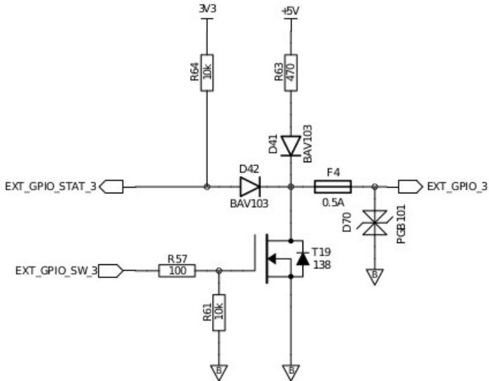
From the schematic above, we can see a 470 Ohm resistor in series with a diode and a 500mA polyfused going to the GPIO port. A max current of approx. 100mA is therefor available for connecting a small relay or an LED. TVS diode D70 protects against electrostatic discharge (ESD).
