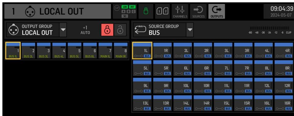
Changing the output routing is made from the **ROUTING**→**OUTPUTS** screen, with first clicking on the **OUTPUT GROUP** of interest to select the first physical destination you want to assign a WING signal to.
