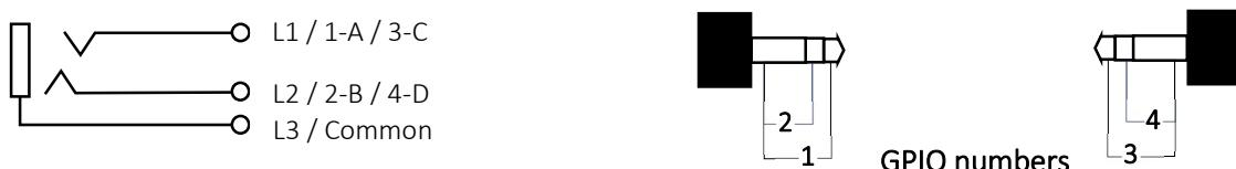
WING GPIO 'mode' settings can be any of the following: TGLNO, TGLNC, INNO, INNC, OUTNO, OUTNC. These are represented by OSC patterns `/$ctl/gpio/1..4 mode`, and correspond to:
