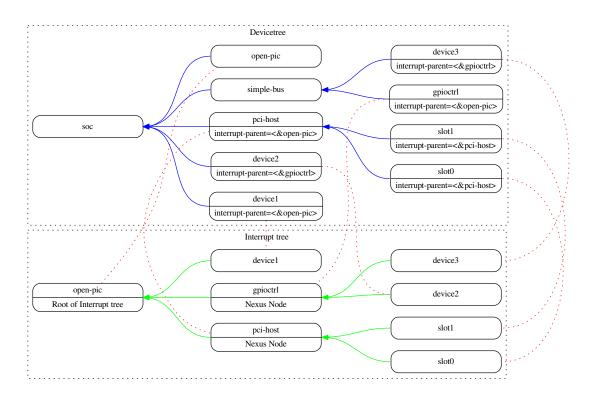
Fig. 2.3: Example of the interrupt tree
